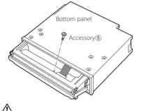
Never insert the screw in any other screw hole than the one specified. If you screw them in another hole, it will contact and may cause damage to the mechanical parts inside the unit.
